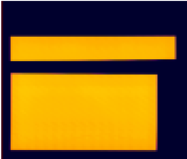
Picture 3: Example of glass sheets recorded with Optris Glass Tempering Scanner (GTS).
