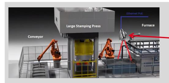
schematic of the installation of thePI 1ML camera
